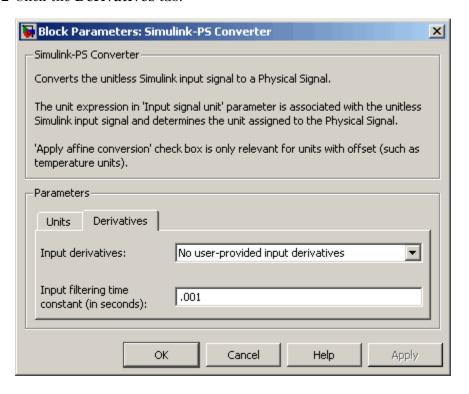
**3** To avoid filtering the input signal, set **Input derivatives** parameter to First derivative of input user-provided.
