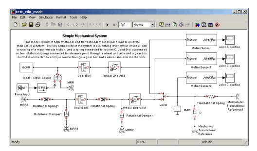
**2** Open the Joint C Position scope and simulate the model.
