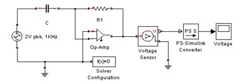
Simulate the model, and you will see that the output is minus the derivative of the input sinusoid.
