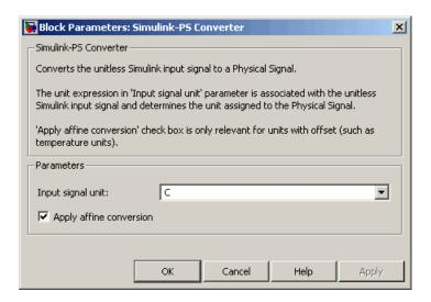
As a result, the Simulink-PS Converter block outputs a value varying between 277 K and 293 K.
