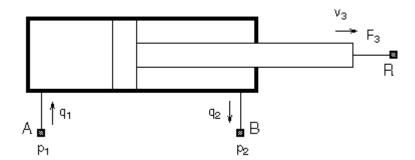
The element is represented with three energy flows: two flows of hydraulic energy through the inlet and outlet of the cylinder and a flow of mechanical
