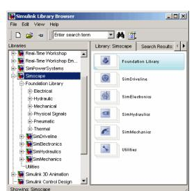
Alternatively, you can type simulink in the MATLAB Command Window. Then expand the **Simscape** entry in the contents tree.
