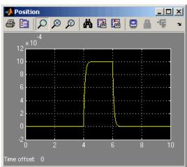
In the beginning, the mass is at rest. Then at 4 seconds, as the input signal changes abruptly, the mass velocity spikes in the positive direction and gradually returns to zero. The mass position at the same time changes more gradually, on account of inertia and damping, and stays at the new value as long as the force is acting upon it. At 6 seconds, when the input signal changes back to zero, the velocity gets a mirror spike, and the mass gradually returns to its initial position.
