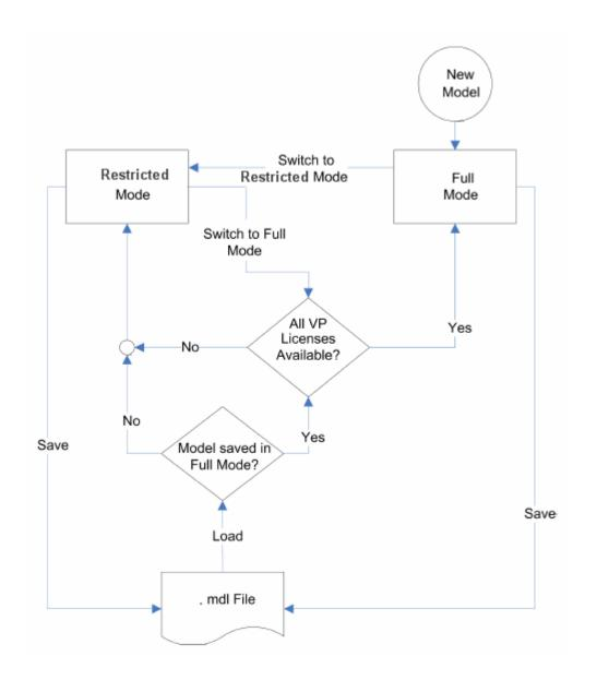
New models are always created in Full mode. You can then either save the model in Full mode, or switch to Restricted mode and save the model in Restricted mode.
