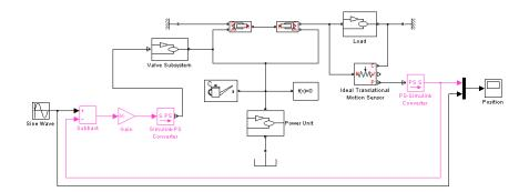
A better way to avoid an algebraic loop without introducing additional dynamics is shown in the modified model below.
