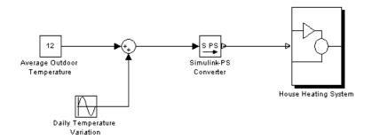
This signal is an absolute temperature reading. Therefore, when the signal converts into kelvin for further computations, you need to specify that it should use affine conversion. Double-click the Simulink-PS Converter block, type C in the **Input signal unit** field, and select the **Apply affine conversion** check box.
